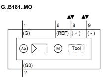
Tool = Configuration and maintenance interface (7-pin)
