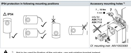
1) Not to be used for fixation of the actuator, use anti-rotation-bracket instead.
